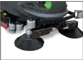
PRE-SWEEP SYSTEM ON CYLINDRICAL MODEL
