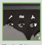
Warning lights Monitor maintenance needs, liquid levels in the tank, and motor activation
